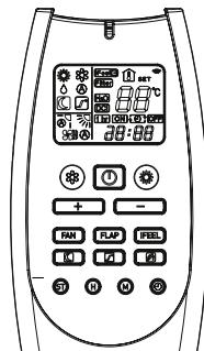
At this point, press contemporary the FAN and IFEEL keys of the remote control for more than 5 seconds and release them by pointing the remote control towards the indoor unit.
