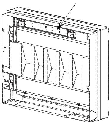
**EG** Remove the fixing bracket from the rear part of the unit.
