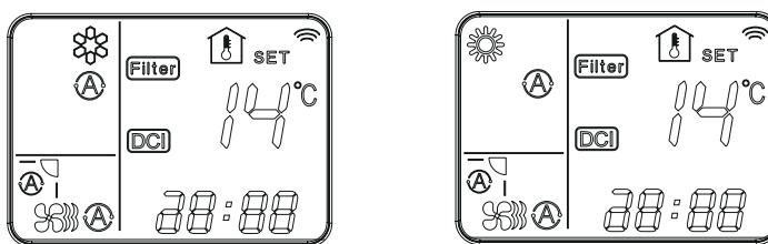
At this point, press together FAN + IFEEL buttons for more than 7 seconds and release them pointing the remote controller to the indoor unit receiver. Be sure to send the signal to only one indoor unit and that there is no other indoor unit that could receive the same signal. If the signal is received, the indoor unit will emit 5 consecutive beeps.
