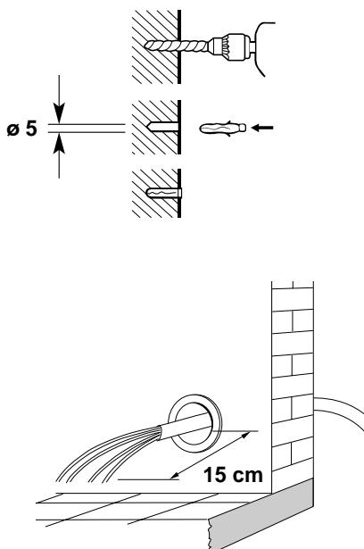
**EG** Make the holes for the fixing of the unit. Running power electric cable (with a ground wire) between the two units (see the table of wire section). Check if the quantity and the rawl plugs type supplied are the proper ones for fixing the unit on the wall.
