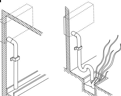
**EG** Install the condensate drain to the outside with a positive slope, form a trap at the end if necessary.
