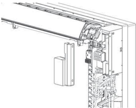
**E** Remove the electrical box cover to operate on the terminal strip.
