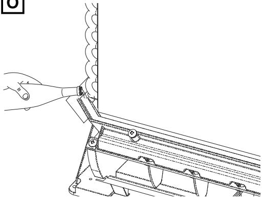
**EG** Fill the tank and verify that the condensate can flow correctly. Reassemble the front panel.
