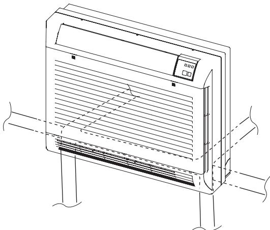
**EG** Find the place for the installation. The unit can be connected in six different positions: at the right-back side, at the left-back side, at the bottom on the right or on the left, on the right or left side.
