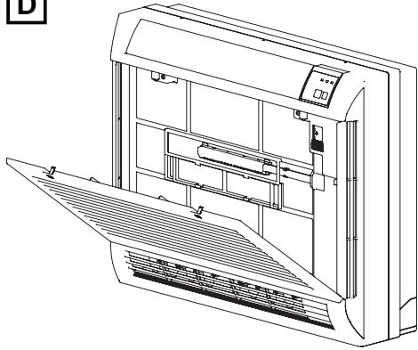
**EG** Before installing the unit it is necessary to remove the front panel:
