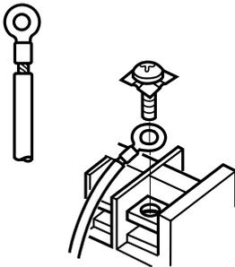
**EG** Predispose the terminals of the wire to connect to the terminal strip, connect them and secure the wiring with clamp provided. (See wiring diagrams).
