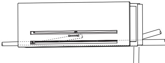
**EG** The unit can be connected to five directions: right rear - left rear - right side - left side and right downward.
