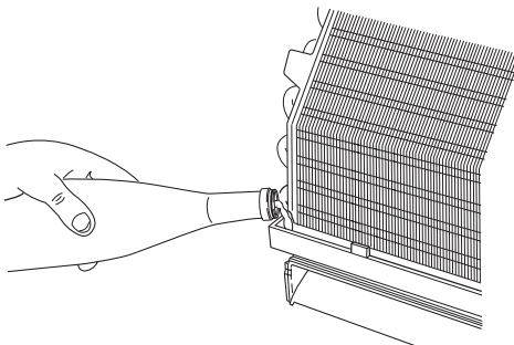
**EG** Remove the front panel. Fill the tube and verify that the condensate can flow correctly. Reassemble the panel.
