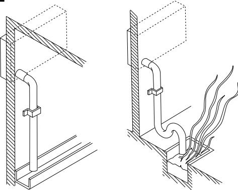
**EG** Install the condensate drain to the outside with a positive slope, form a trap at the end if necessary.
