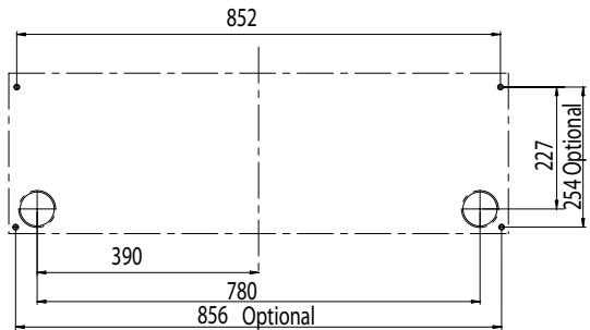
**EG** Tubing connections from the rear. Place the full call diagram, mark the holes to be made on the wall, check the horizontal position with the level (OPTIONAL HOLES).
