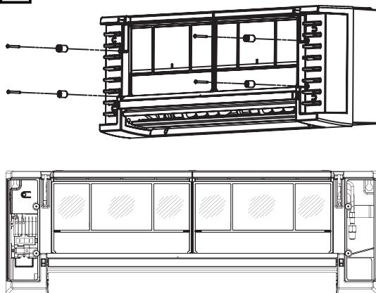
**EG** Remove the cover plates' screws and spacers to reach the hydraulic and electrical connections.
