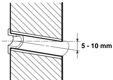
**EG** Drill a 65 mm diameter hole, insert a PVC pipe.
