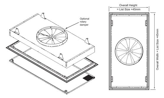
We offer two size options for the PGL2 with a larger unit to suit plaster ceilings and slightly smaller unit to provide an overall size designed to fit regular T bar type ceiling grids.
