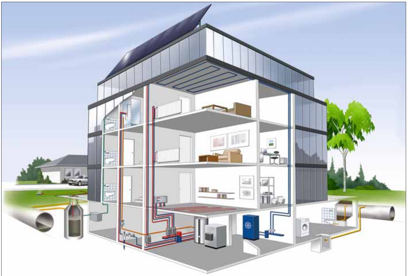
Example: Construction of a solar installation in a one-family house
