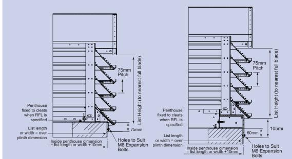
**B1 Border**: Manufactured from a minimum list length of 600mm to a maximum list length of 1900mm Please note width is always equal or less than length
