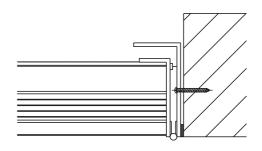
UNIT SECURED WITH M6 EXPANSION BOLTS ON 600mm CENTRES THROUGH OUTER FRAME
