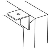
UNIT SECURED WITH M6 EXPANSION BOLTS THROUGH FIXING ANGLE CLEATS MOUNTED AT 600mm CENTRES AT REAR
